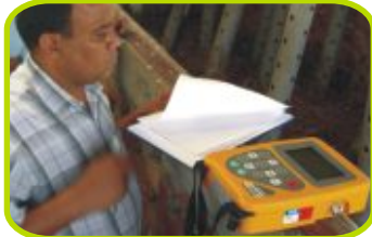
Methane & oxygen monitoring
