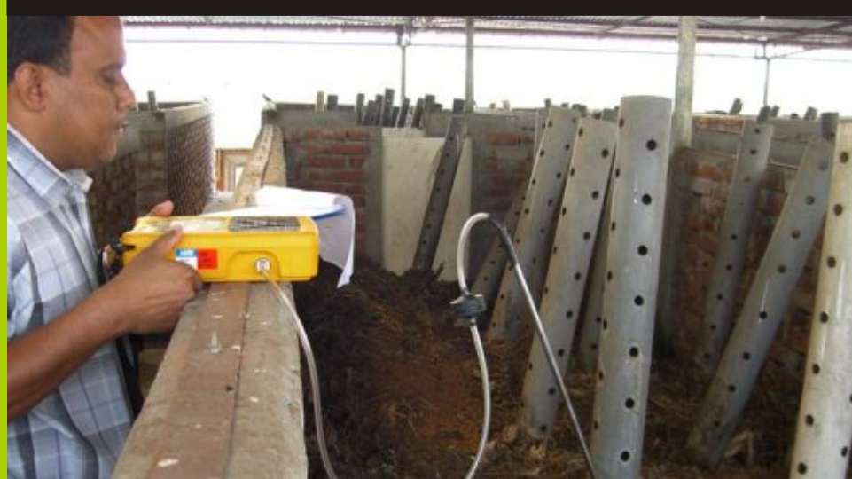
Methane emission monitoring
